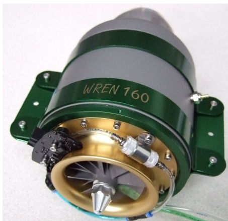
Wren 160 engine "under the covers", showing rpm pcb and fuel filter arrangement
